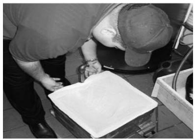
1. Install strainer bag in warmer and place under the grill to collect grease for the day.
