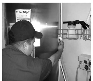
14. Release the hose from the warmer and attach it to the holder on the side of the tank.
