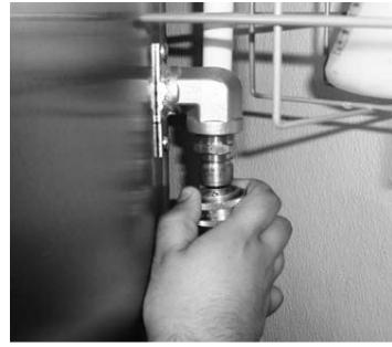
7. Pull the collar back and remove the hose from the holder.
