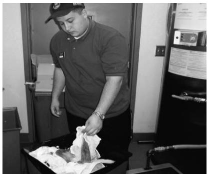
13. Remove the strainer bag and discard it into a lined trash container.
