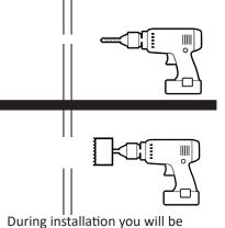
required to Drill a 2.5" hole into the shed. Start with a 1/4" pilot hole through the shed. Then bore a 2.5" hole. Using a Greenlee Slug Buster will provide a clean professional result.
