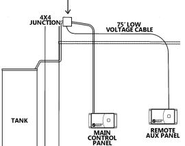
Make the connection INSIDE the junction. Do NOT leave any connectors outside of the junction box. Tighten the wire gland around the 75' cable.
