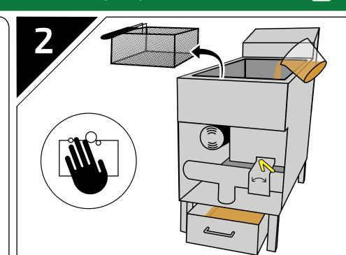
Remove fryer baskets and accessories. Rinse any crumbs from the fryer into the filter pan. Clean the fryer following your company's procedure.
