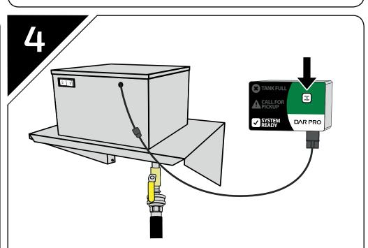
If a push to pump panel is located next to your pump station, start and stop the system by pressing the push to pump button.
