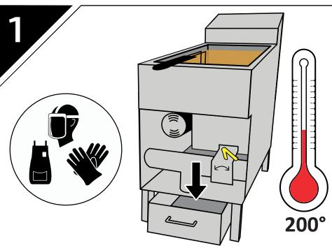
**Remember your PPE!** Turn off the fryer and allow oil to cool. Drain the oil to the fryer's filter pan.
