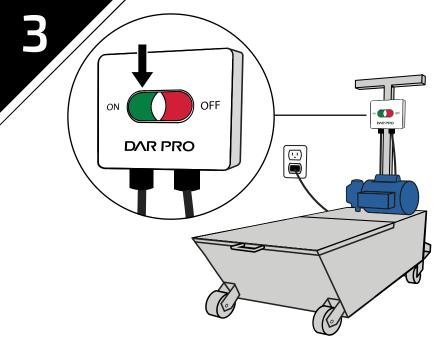
If your caddy has a Push to Pump (PTP) panel, plug the caddy into a wall outlet. Press the green Push to Pump button to discharge the oil.
