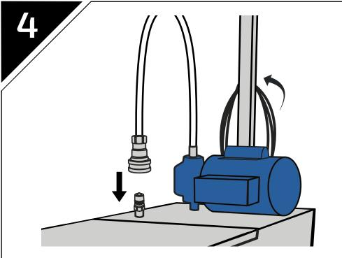
Once all of the oil has discharged from the caddy, reconnect the hose and coil the cords.
