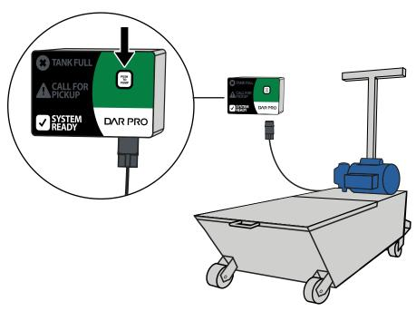
For a non-PTP caddy, connect the caddy cord from the motor to the tank control panel. Press the Push to Pump button to discharge the oil.
