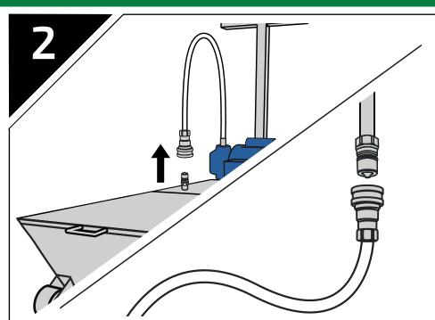
Remove the female quick disconnect from the caddy by pulling back on the collar. Connect the hose to the tank fill line.
