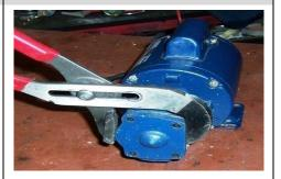
Remove end cover by rotating back and forth or tapping from the back of the cover.
