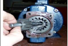
Lubricate the pinion assembly with gear lube or cooking oil and reinstall.
