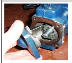
Reinstall the end cover. It should slide on without forcing. If it will not install easily, make sure the pinion assembly is seated into the motor shaft.
