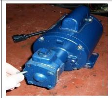
Reinstall the end cover bolts. Do not over tighten as this will bind the pump.
