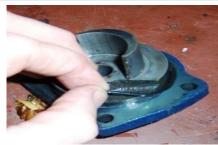
The end cover has a seal called a square ring. Do not lose or damage this seal. If it is damaged, replace it.
