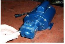
Loosen and remove the end cover bolts.
