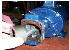
Lubricate the rotor with gear lube or cooking oil and reinstall.
