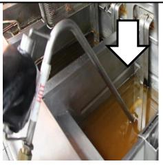
Insert the Wand into the Fryer. Hold the Wand until as much oil as possible is removed from the Fryer.
