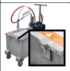
Turn the Motor OFF, unplug the caddy, and return the Wand to the holder. Ensure the Caddy Lid is SHUT and SEALED before transporting.
