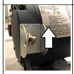
Turn on the Caddy Motor ON and remove the wand from the holder.
