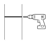
Drill a 1/4" pilot hole through the exterior wall. Before drilling always check the wall for electrical, plumbing or any other obstructions.
