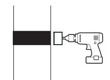
Using the pilot hole, bore a 2.5" hole halfway through the wall from the inside of the building, then complete the hole from the outside, meeting in the middle of the wall. This will reduce chipping of the wall surface.
