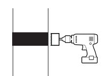
Using the pilot hole, bore a 2.5" hole halfway through the wall from the inside of the building, then complete the hole from the outside, meeting in the middle of the wall. This will reduce chipping of the wall surface.
